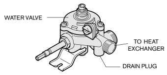
Fig. 0 - Water heater drain plug
